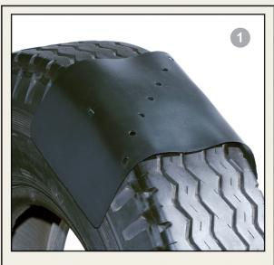
Place Wick Pad on the opposite side of the tread joint and far from repaired areas. Adjust it to tyre shoulder.
